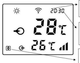
1. Hours flashing, press + or - to set the hour.
