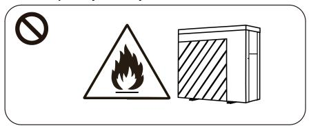
b. The installation can't be in a closed environment or indoors, and must be kept well ventilated.
